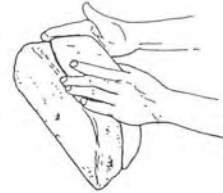
70. Press clay to fill the mould.
