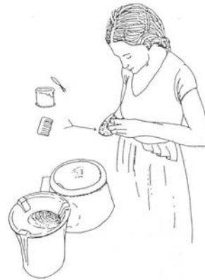
84. Score and slip the back of the potrest.
