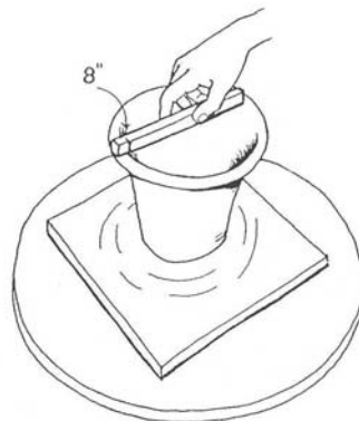
68. Measure the inside width at the top – it should be 8".
