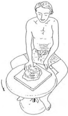
4. Slap clay onto the pallet while turning the wheel.
