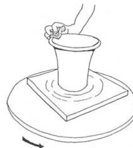
69. Sponge the rim, widening or narrowing the width as needed.
