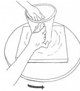
63. Continue up the wall, removing excess clay and shaping the wall. Clean the rib as needed.
