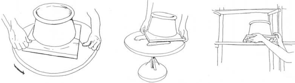
30. Use a piece of string to cur the firebox from the pallet.
