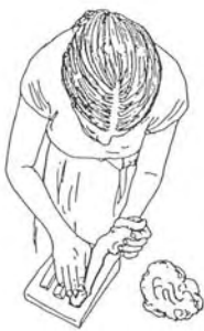
47. Press clay into the buttress pressmould.
