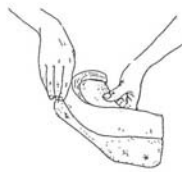
72. Remove excess clay from the top and sides.
