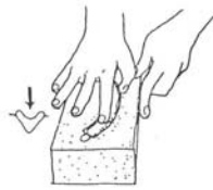
58. Using a fingertip, press a curved indentation that is level with the indentations in the plaster at the edges of the arc shape.
