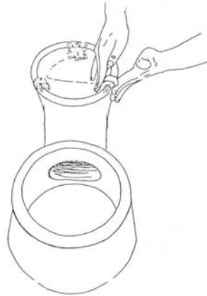
45. Use two hands to press the potrests firmly in place. The short flat side should be horizontal on top.
