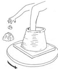
18. Remove excess clay from the inside bottom again.
